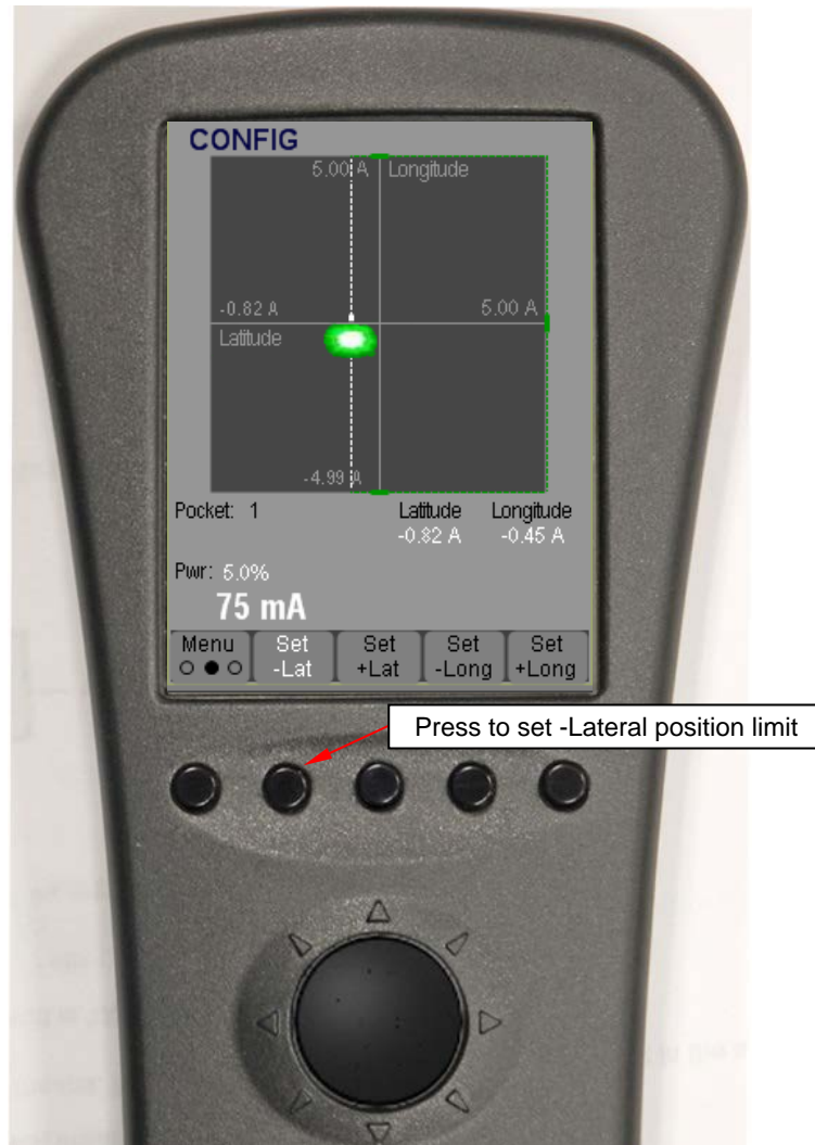
Figure 20 Remote Controller in Config Mode with Menu 2 Selected, User Setting the -Lat Position Limit
