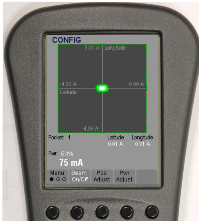
Figure 18 Remote Controller in Config Mode with Menu 1 Selected and Beam on at 5%,
