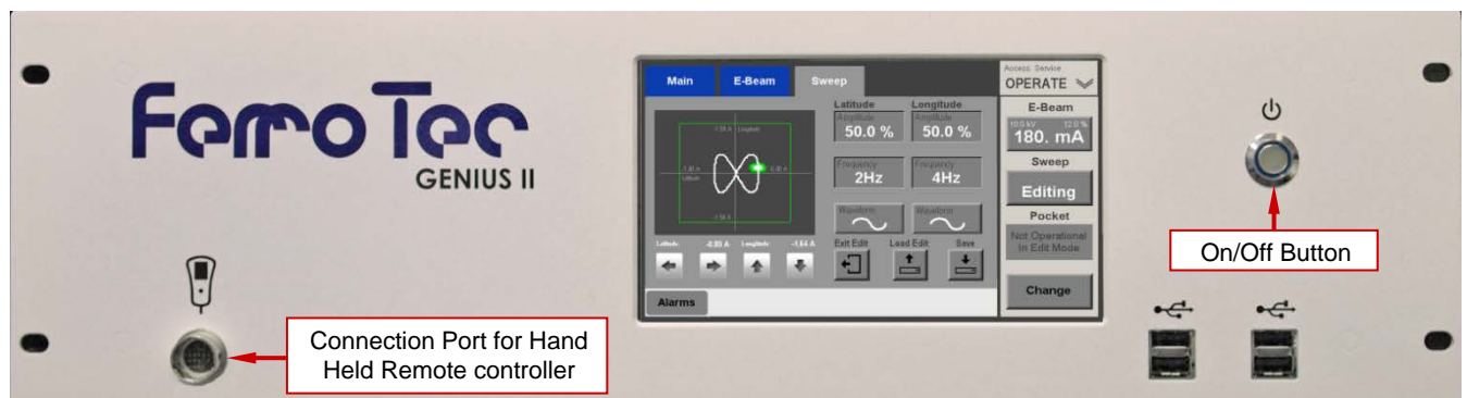
Figure 1 Genius II Front Panel, Showing Connections Port for Hand Held Remote Controller
