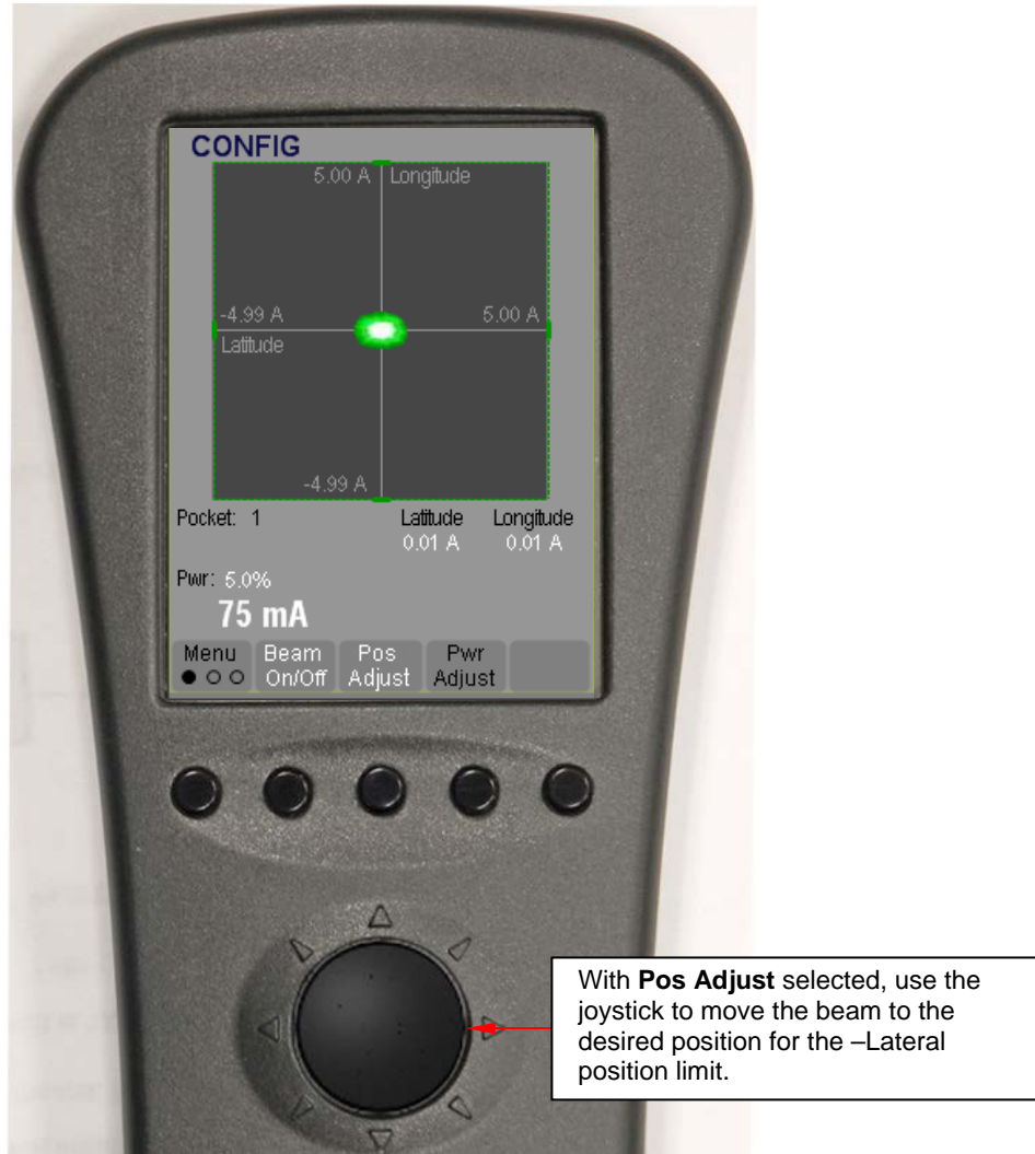
Figure 19 Remote Controller, Beam On @ 5%, Config Mode, Menu 1 and Pos Adjust Selected
