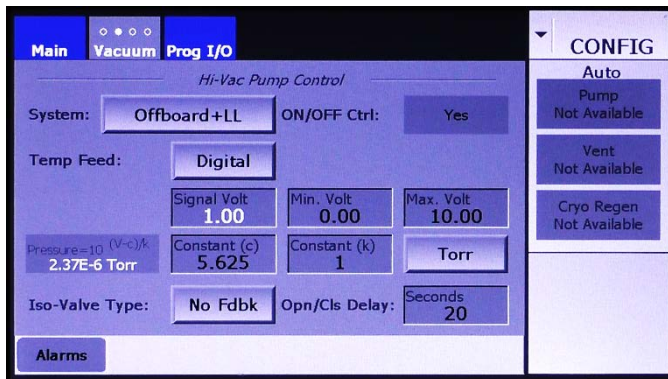
Figure 10-4 Hi-Vac Control Page After User Selects No Fdbk
