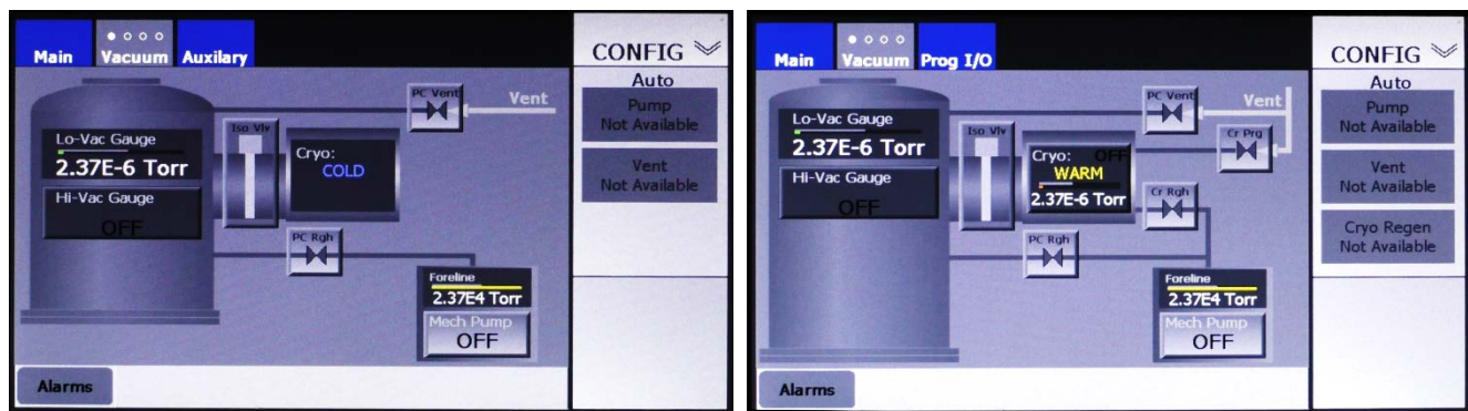
FerroVac Configured for an On-Board Cryopump
