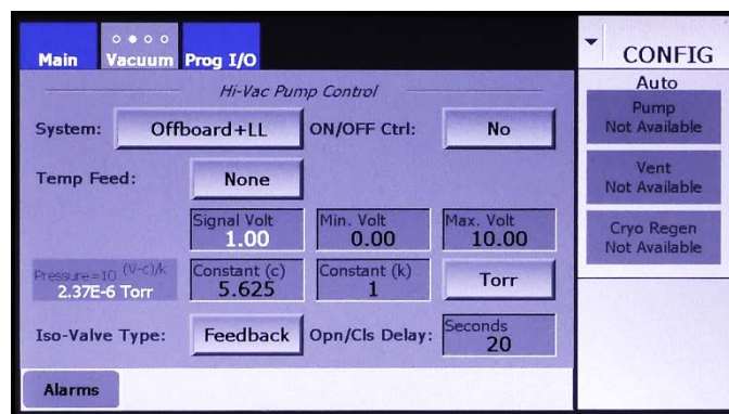
Figure 10-35 Cfg>Hi-Vac Pump Control page: None Selected for Temp Feed, No for On/Off Ctrl
