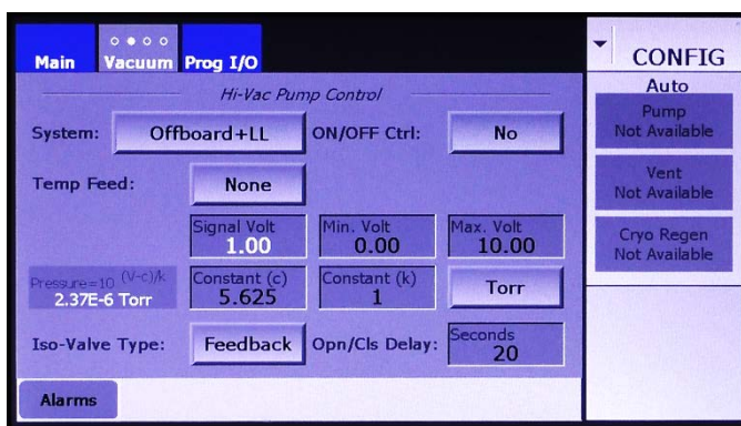
Figure 10-3 Hi-Vac Pump Control Page: None Selected for Temp Feed, No for On/Off Ctrl
