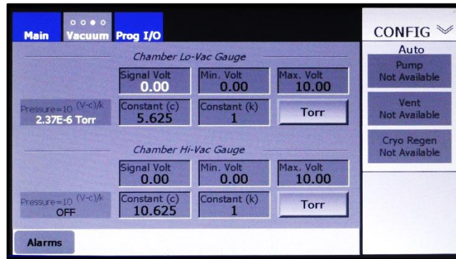
Figure 3-11 Config>Vacuum Screen, Page 3 (Chamber Vacuum Gauges Page)
