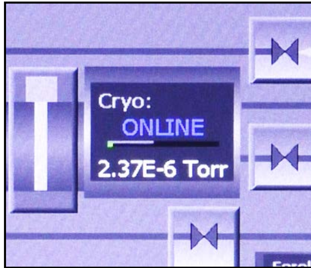
Figure 6-14 Vacuum Map's Cryopump Icon when None Is Selected for Temp Feed , No for On/Off Ctrl
