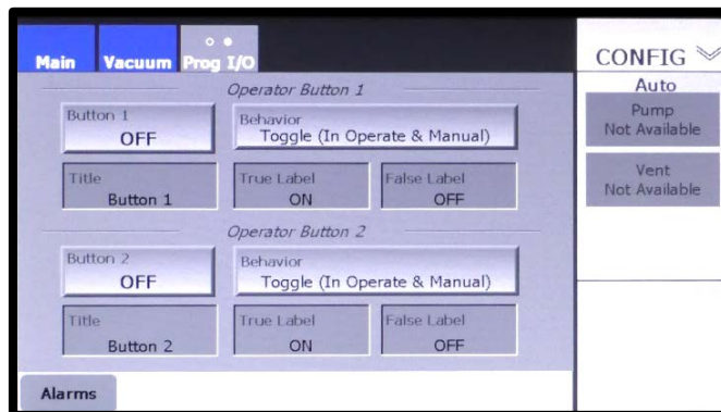
Figure 4-21 Prog I/O Screen, p. 2: Outputs Assigned to Both Buttons, Neither Configured
