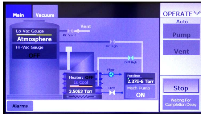
Figure 8-13 Ops Mode Vacuum Map After User Starts Autopump
