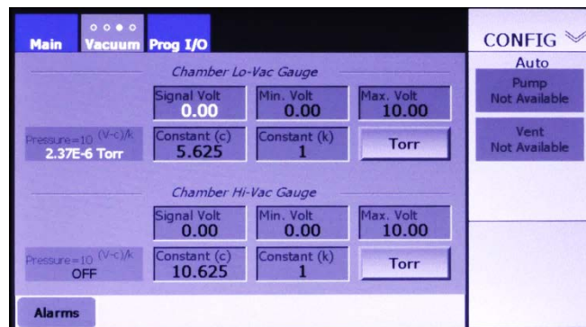
Figure 4-6 Chamber Vacuum Gauges Page at Initial Boot-Up
