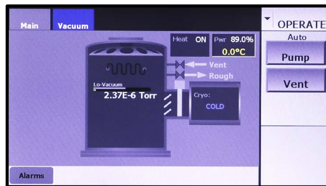
Figure 12-29 Ops>Main Screen: Configuration State 2 Implemented, Operate Mode SP = Operator Control
