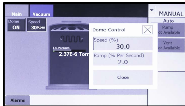
Figure 11-12 Dome Control Popup as Displayed when Enable User Set Ramping = No
