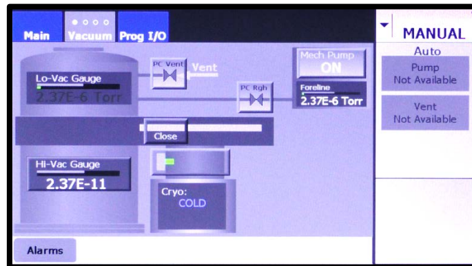
Figure 9-8 Vacuum Map when Nonzero Values Are Entered for Roughline Purge and PC Soft Rough
