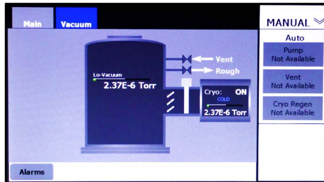
Figure 6-5 Manual>Main Screen when None Is Selected for Temp Feed , Yes for On/Off Ctrl
